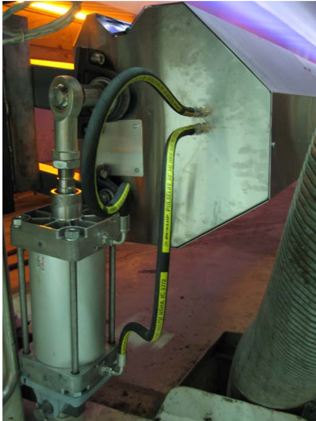
Inspection beam mechanics at the operator side. Pneumatics tubes emerge from the beam and are connected into the pneumatics cylinders, which enable up / down movement of the inspection beam e.g. in order to facilitate paper tail threading.
